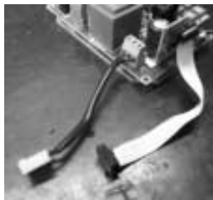
The inverter is supplied with power and logic connection cables for the KS card.
