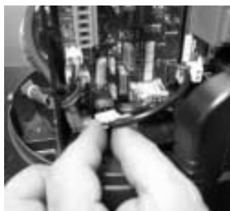
Insert the capacity connector of the inverter on the KS
