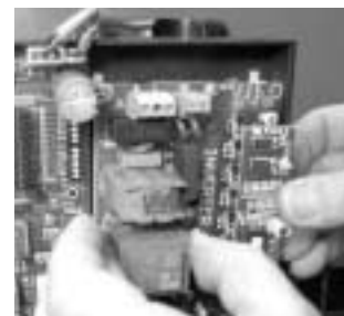
Insert the inverter onto the 4 spacers.
