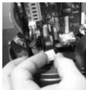
Remove the protecting connector on the KS.
