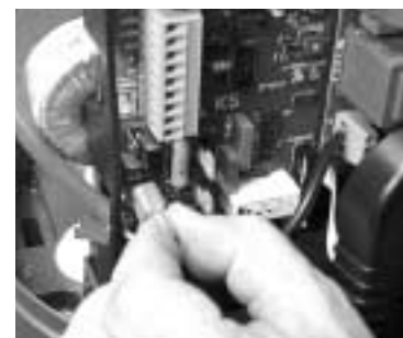
Disconnect the motor cables from the KS
