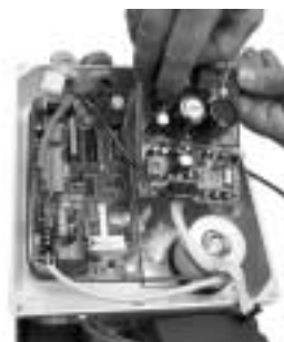
Insert the inverter onto the 4 spacers.
