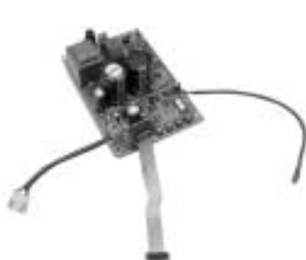
The inverter is supplied with power and logic connection cables for the KS SUPER
